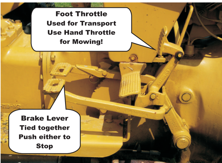
Figure 6 Brake and Foot Throttle Pedals
